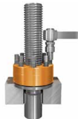
Very long through stud A special tensioner with a larger circle of jackbolts may be necessary to properly access the jackbolts for tightening.
