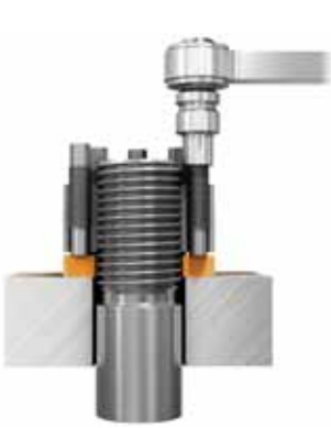
Centering of washer on thread Make sure the washer is not resting on one side of undercuts or radius of mating studs.
