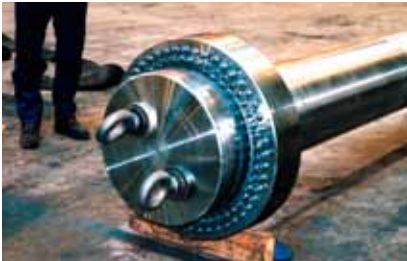
The world largest bolt-style multi-jackbolt tensioner 28" diameter x 40' long (711,2 mm diameter and 12,2 m long). This was used on a large hydraulic forging press.
