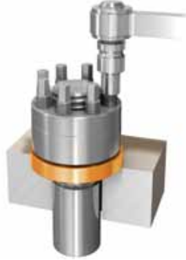
Material with low strength A thicker / larger washer or an additional washer may be necessary when materials with low strength are used on the joint.
