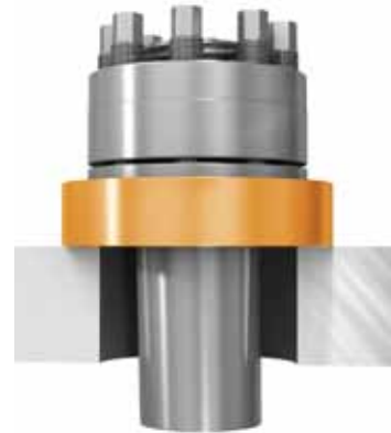
Large or slotted holes An additional washer or a large washer is necessary to transfer the bolt load to a supported surface.
