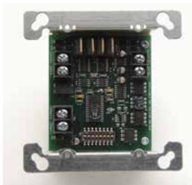
The 4090-9117 Power Isolator provides monitoring and short circuit protection for 24Vdc power wiring to IDNet addressable devices. In the event of a short circuit, it opens a two-pole electronic switch, isolating both power circuit conductors. This function can also be selected from the CIE. The isolator reports to the CIE, when it is in isolation mode. It also reports the extent of shorted wiring by identifying the addresses of non-communicating devices
