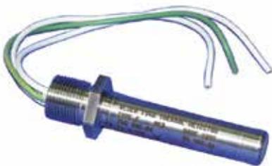
T54B is a simple device and therefore suitable for use in intrinsically safe areas when used with a suitable I.S. barrier. For reliable operation, it is recommended that T54B detectors have set points 20°C or 20% (whichever is higher) above the maximum temperature they will be exposed to in normal operation. Preferred factory preset temperatures range from 60° to 250°C; with normally open contacts. Other temperatures and normally closed contacts are available by request.
