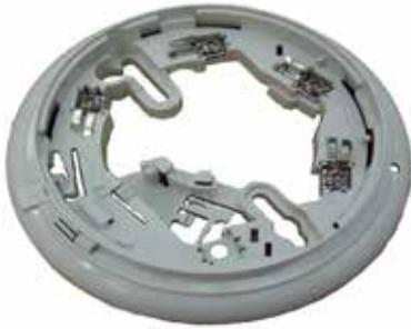
The 5B Universal Base contains no electronics and is suitable for indoor applications of both the 614 series collective (non-addressable) and 814 series analogue addressable detectors. It provides excellent space for cable access and terminations. Its larger skirt makes it suitable as a replacement for the earlier M614 base to cover any paint rims or for covering a larger hole in the ceiling. It features remote LED connections and an anti-tamper facility.
