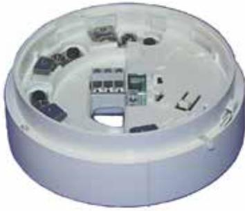
The 814RB Addressable Relay Base provides two sets of changeover volt-free relay contacts capable of switching 1A (resistive) @30Vdc. The relay function is controlled by the *MX* fire alarm panel via the detector fitted to the 814RB. The 814RB may be mounted to the ceiling, plugged into an M6 14/5B Universal Base or an 5BI/8 14IB Isolator Base.
