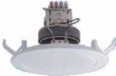
The 'One Shot' PA speaker and grille is designed to install easily into 10 to 13mm gyprock/plaster/acoustic ceilings. Simply drill the required size hole, terminate the wiring and push the speaker into the ceiling until it snaps into place. They are designed to meet the requirements of AS2220.1, with a transformer cover (not shown in the image) and 22µF capacitor. The transformer has 5 power taps from 0.33 to 5W and a 4 way terminal block.
