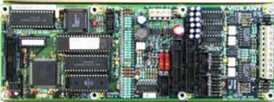
The Panel-Link Modbus Bridge (PMB) is designed to translate data from VIGILANT fire alarm systems on a Panel-Link network to a Modbus communication line. The PMB not only monitors the Panel-Link network, but also provides a means of direct control over the fire systems. The PMB database contains data on the
