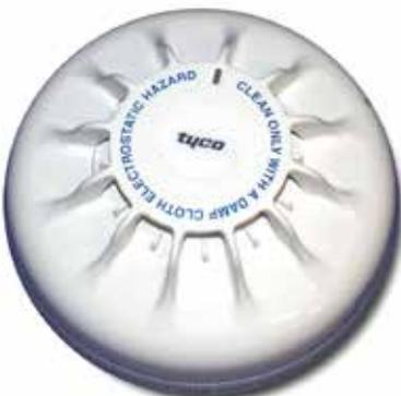
The 801HEX Intrinsically Safe Heat Detector forms part of the 800Ex Intrinsically Safe Series of *MX* Addressable Fire Detectors. The detector plugs into a 5BEx base. The detector is designed to transmit to a remote *MX* fire controller, digital signals which represent the status of the heat element of the detector. Software within the controller is used to interpret the returned heat values to raise an alarm or other appropriate response according to the programmed configuration.
