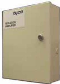
The FP0875 Isolation Amplifier connects to an existing 100V speaker line and reproduces this signal at up to 50W load on a separate supervised 100V line. It is suitable for use with speech and music as well as with warning tones. The 100V output line from the amplifier is electrically isolated from the input 100V line, so noise or other signals on the output line are kept separate and do not affect the input line.
