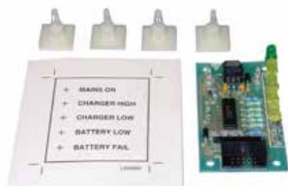
This PCB Assembly connects via a flat ribbon cable to the PSU24XX range of power supplies. The PCB provides optional Mains On, Charger Low, Charger High, Battery Fail and Battery Low LED indicators which may be mounted on the front facia of equipment. PCB Dimensions (mm): 75H x 40W x 3.0D. Supplied complete with self-adhesive PCB stand-offs and LED label. It mounts on 4 adhesive-based stand-offs, included with the PCB. Five Ø5.5-6mm holes need to be drilled at 10mm vertical spacing for the LEDs.
