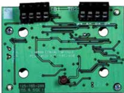
The CIM800 Addressable Contact Input Module monitors and supervises two circuits of voltage-free contacts such as outputs from extinguishing systems, ventilation controls, fire door controls,
