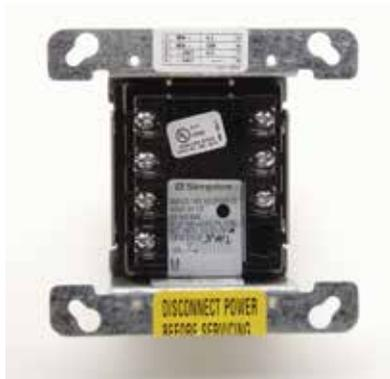
The 4090-9119 allows a 4100ES IDNet communication channel to monitor an unsupervised input contact with one point and control an output relay with the other point, yet occupy a single address. The input circuit and relay operation are controlled independently and may be disabled separately. Module power is supplied from the IDNet communications channel eliminating the need for separate power wiring. The address is set by DIP switch under the re-sealable label.
