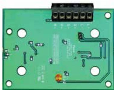
The LIM800 Line Isolator Module is designed to be used on the MX addressable controller loop circuits. It monitors the line condition and when detecting a short circuit will isolate the affected section whilst allowing the rest of the addressing circuit to function normally.
