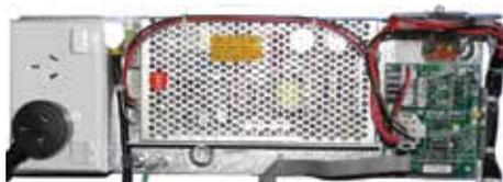
The 5A ME0476 Power Supply is a direct replacement for older 2.5A FP0874/FP0825 supplies. The ME0476 is used in MX4428 panels (or F4000 upgraded to V3.10+ software).
