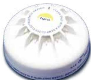
The MDU601EX detector combines the features of both the MU601EX detector and the MD601EX detector to provide a combined CO and Rate of Rise Heat Detector where the sensitivity of the CO detector is enhanced in response to a fast rate of change of temperature.
