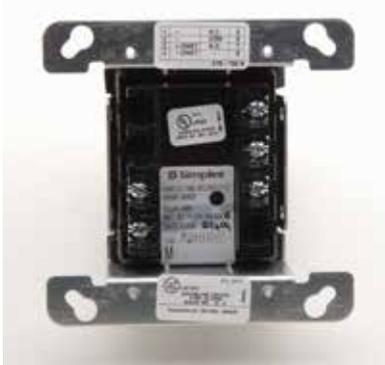
The 4090-9002 Relay IAM allows the CIE to control a remotely located Form "C" Relay contact using IDNet addressable communications for both data and module power. Typical applications are for switching local power for control functions such as magnetic door holders, or control of HVAC components, pressurisation fans, dampers, etc.. Relay contact status is also communicated to the CIE. The address is set by DIP switch under the resealable label.
