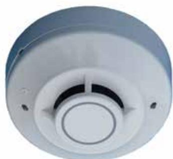
The T131A-Mk2 heat detector is a state-of-the-art dual thermistor heat detector with analogue communication electronics. Used in conjunction with the VIGILANT MX4428 panel, the T131A-Mk2 has a high degree of false alarm immunity thanks to the advanced SmartSense algorithms. It is panel programmable to either Type A (with Rate Of Rise) or Type B (fixed temperature only) to maximise system design flexibility.
