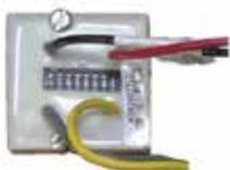
This IDNet addressable device is an encapsulated version of 4090-9001. It has both power and communications supplied by a two-wire IDNet circuit. It provides location specific addressability to a single initiating device (such as single station smoke detector alarm contacts or heat detector contacts) or multiple devices at the same location by monitoring normally open dry contacts and the wiring to an end-of-line resistor.
