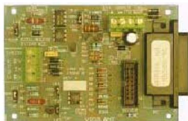
The RZDU to RS232 Interface is a small printed circuit board that converts Remote Zone Display Unit serial communications from a fire indicator panel into RS232 compatible signals. This module is required for an IO-NET Controller to receive information from an F3200/MX4428/F4000/MX1 fire alarm panel.
