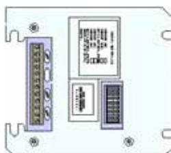
Monitor ZAMs are used when the fire detecting devices or supervisory switches are mounted separately from the addressable electronics. It provides status monitoring and supervision to the device circuit zone and is used for circuits with non-addressable detectors and for other contact closures eg., waterflow and tamper switches or non-addressable manual stations.
