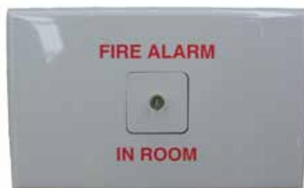
The E500 Mk2 range of latching remote indicators provide latching remote indication of an alarm condition on a fire detector. They are used typically where a T54B probe type fire detector is installed (which may be in an inaccessible location), and indication of alarm must be provided in an easily accessible area. For example, where the detectors are in roof spaces or cupboards, exhaust hoods etc and indication is required in the room or corridor.
