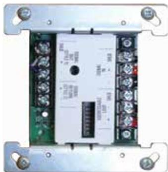
This IDNet addressable device provides a supervised, addressable interface to conventional warning devices such as sounders or strobes. The Signal IAM requires a supervised power supply or compatible signal input for powering the externally connected loads.
