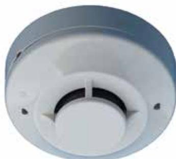
The P131A-Mk2 photoelectric smoke detector contains a state-of-the-art sensing chamber and analogue communication electronics. Used in conjunction with the VIGILANT MX4428 panel, the P131A-Mk2 has a high degree of false alarm immunity thanks to the advanced SmartSense algorithms.
