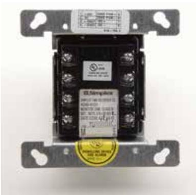
The 4090-9101 Zone Adaptor Module Monitor ZAM allows a 2-wire circuit of collective smoke or heat detectors to be interfaced on to the IDNet loop. Up to 20 collective heat and smoke detectors can be monitored by a 4090-9101 Monitor ZAM. The address is set by DIP switch under the re-sealable label.
