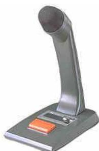
The SU0169 Paging microphone is a desktop dynamic microphone with a cardioid polar pattern. It features a short-off press to talk switch with an open-off type extra switch. It has low handling noise and a 600 ohm balanced output impedance. Compatible with the FP0539 Paging Console.
