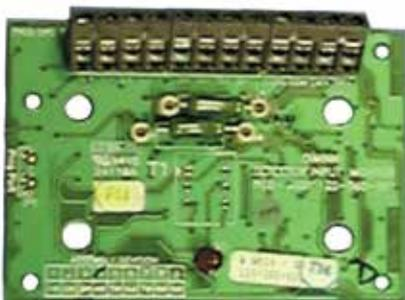
The DIM800 Detector Input Module interfaces two collective detector circuits onto the *MX* addressable loop.
