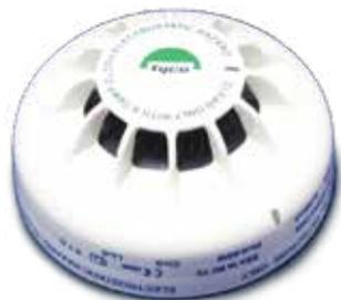
The MR601TEX has been developed to overcome the slower response of the optical detectors to hot burning fires, by increasing the sensitivity of the optical detector when it is associated with a rapid change in temperature. In this way it is intended to become a detector which can cover some of the risks currently covered by ion chamber detectors. Smoke detectors will not detect burning alcohol or other clean-burning liquids which do not generate smoke particles.
