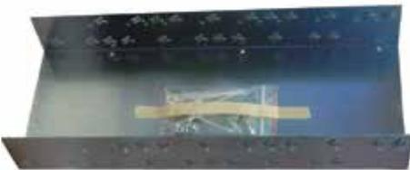
A KT0072 Cardframe upgrade kit can be fitted to a 15U F3200 to allow it to take more than three 8 way modules. The KT0072 cardframe can accommodate 8 F3200 modules (for MX4428:- 8 ADR or 6 MPR/MXP/ADR+RRM). In older versions, the cardframe mounts directly to the rear of the cabinet. In newer versions, the cardframe is fitted to a gear plate that may be removed when the cabinet is mounted to the wall.
