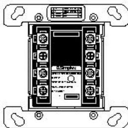
The 2190-9173, 2-Point I/O module allows a Simplex MAPNET II communication channel to monitor an input contact closure and control an output relay from a single compact module. Module power is supplied from the MAPNET II communications channel. The monitor and control points can be applied for a variety of associated or independent operations. Flexible programming abilities at the host panel can provide the association logic required for a wide variety of fire or utility operations
