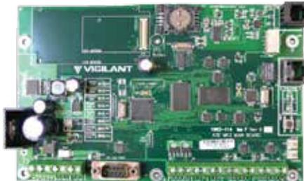
Configuration and diagnostics are performed from a standard PC web browser anywhere on the network. The PIB also provides remote across-network access to the diagnostic port of any panel directly connected to a PIB. It is supplied complete with Ethernet, MX4428 serial port, and IHUB/panel FRC network port looms.
