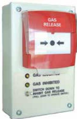
**FP0570** Local Gas Control Station - Automatic. Local Gas Control Stations (LGCS) are used in gaseous fire extinguishing systems to provide local area manual control of a release. The automatic version includes a Gas Inhibit switch, buzzer and LED, whereas the manual version (FP0572) does not. The LGCS is fitted with a resettable no-break plastic frangible element.
