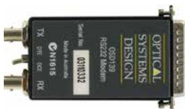
The OSD139AF Asynchronous RS232 Transceivers can interconnect one RS232 data channel over 3km of multimode fibre (OSD139AF) or over 50km of singlemode fibre (OSD139AFL). These can provide complete end-to-end isolation of a full duplex asynchronous data transmission at up to 60kbps.
