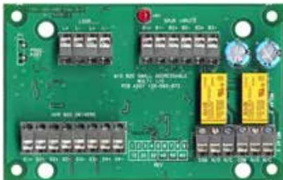
The MIO800 Multi-Input Output Module allows multiple input and output connections to be made between external equipment and the *MX DIGITAL* loop. Three inputs and two outputs are provided. Each input and output can be programmed independently to provide customised functionality. An IP55 rated D800 style housing can be used as the standard enclosure, with the option of a DIN-rail mounting kit for in-cabinet installation.
