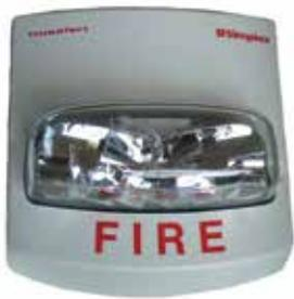
The 4906-910x Multi-Candela strobe is a high output xenon strobe capable of signalling evacuation using the ISO 8201 "T3" temporal pattern, as required by AS 1670.4-2004 and AS 1670.1-2004. It produces white light with a link-selectable intensity of 15cd, 30cd, 75cd or 110cd. It is controlled by either the ISO 8201 Strobe Driver Module (PA1043) or a QE90 STRM Strobe Relay Module (PA0697). Note: A 24V output cannot be used directly.
