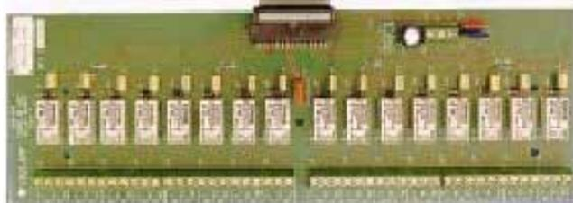
The 16-Way Relay Board has the same physical dimensions and footprint as the 32-Way Protected Termination Board. It comes complete with a 1.4 metre 26-way flat ribbon cable (LM0056) for connection to one of the IO-NET output connectors.
