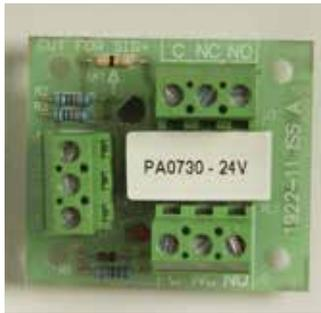
The 24V PA0730 two pole changeover contact general purpose relay board may be used in either of two modes:
