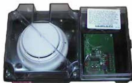
The TrueAlarm duct sampling unit detects the presence of smoke in air conditioning or ventilating ducts. Sampling tubes are installed into the duct and air is directed to a 4098-9714EA smoke sensor mounted in the housing.
