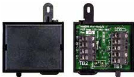
The MIM800 Mini Input Module monitors a voltage-free contact and transmits its state to the c.i.e. It can be programmed to monitor either Normally Open (default) or Normally Closed contacts. The MIMs can be programmed to monitor:
