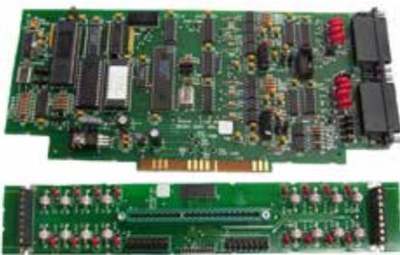
SIMPLEX/VESDA High Level Interface (HLI) allows SIMPLEX addressable fire detection panels to gather and process status information from VESDA LaserPLUS and LaserSCANNER high sensitivity air aspiration smoke detection systems. Hardware requirements include an Intelligent Interface Module installed in the fire alarm control panel and an HLI Module installed in the VESDA smoke detection equipment.
