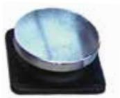
The EA0411 Electromagnetic Door Holder is designed to hold fire and smoke doors open under normal conditions, but automatically close under their own spring return mechanism when a fire or smoke alarm system is activated. The door is held open by the magnetic force between an
