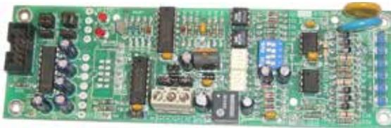
**PA0773** RS485 Comms CMOS PCB 1901-139-3 FRC only (FRC connection - including power). The PA0773 is used to interface an F3200 FIP, MX4428 FIP, PTM, NLDU, MODBUS BRIDGE, RDU or NDU with the RS485 network. This RS485 Communication Board is mounted on four metal stand-offs, which are used for earthing the PCB. This RS485 board connects to the controller board via a 10 way FRC LM0172 (ordered separately), which is also used to power the RS485 Board.
