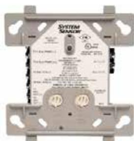
The ADCS130-Mk2 Supervised Relay Control Module provides a single switched supervised output on the MPR addressable loop. It supervises the output wiring for open or short circuit faults when the output is de-energised. The ADCS130-Mk2 can directly replace an ADC130 configured for supervised output operation (tabs in place).
