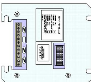
Signal ZAMs are used to supervise and operate 24 Vdc notification appliances, speakers, and telephone circuits. Output capacity is up to 2 A @ 24 Vdc, or 50 W of 25 VRMS speakers, or up to 3 simultaneously activated firefighter phones. The signal ZAM is available for either Style Y/Class B or Style Z/Class A operation for notification appliance circuits.
